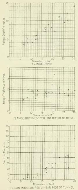
Fig. 42.—Cast iron linings in waterbearing ground. Relationship between diameter of tunnel and flange depth, flange thickness per linear foot of tunnel and section modulus per linear foot of tunnel.
