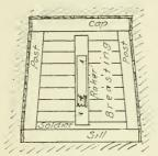
Fig. 1.—Square set headingin dry ground. Cross section.
