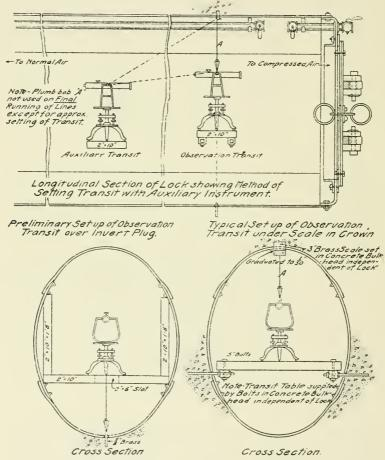
Fig. 159.—Methods of setting transit in air-lock.
