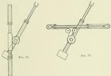
Fig. 73.—An erector turned by rack and pinion. Turning jacks vertical. Fig. 74.—An erector turned by pulleys and chains. Turning jacks horizontal.
