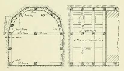
Fig. 3.—The American system of tunnel timbering.
