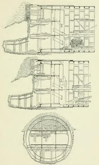
Fig. 124.—Work in mixed face with sliding hood. Pennsylvania Railroad East River Tunnels (A-19). (From  $Trans.\ Am.\ Soc.\ C.\ E.$ , vol. 68.)
