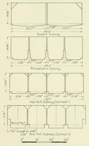
Fig. 8.—Cross sections of rapid transit subway tunnels.
