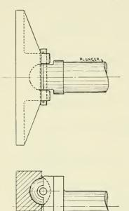
Fig. 68.—Shield jack equipped with ball and socket joint.
