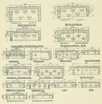
Fig. 41.—Cast iron linings in waterbearing ground—cross sections.
