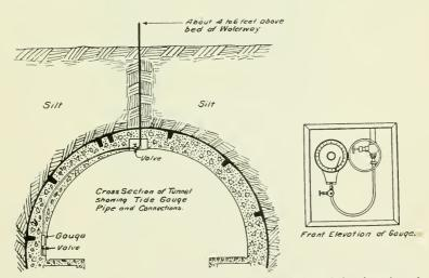
Fig. 136.—Recording gauge for showing the tidal variation of the elevation of the surface of the water above a tunnel in mud.
