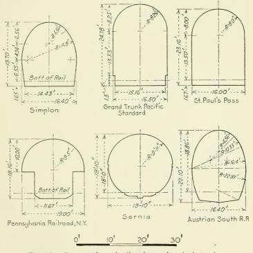
Fig. 10.—Cross sections of railroad tunnels—single track.
