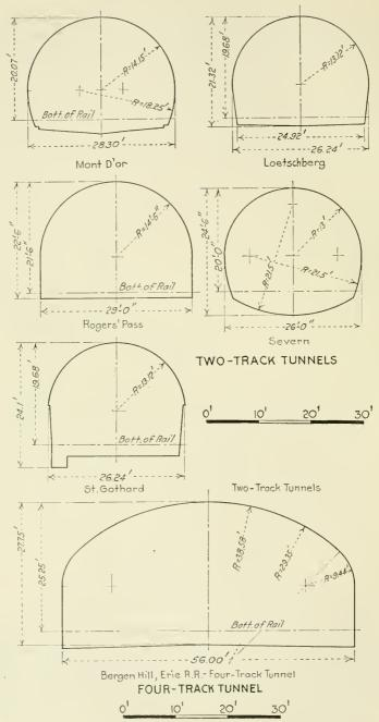
Fig. 11.—Cross sections of railroad tunnels—two- and four-track.
