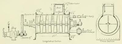
Fig. 93.—Greathead type of grouting machine driven by compressed air engine.
