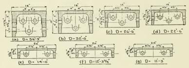
Fig. 39.—Cast iron linings in London clay, cross sections.
