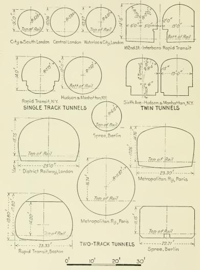
Fig. 7.—Cross sections of rapid transit railroad tunnels.
