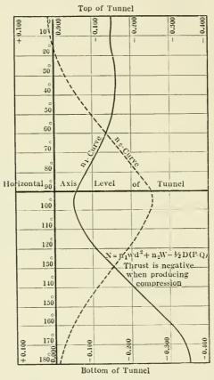
Fig. 26.—Values of constants n<sub>1</sub> and n<sub>2</sub> for all points of the circumference.
