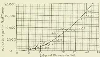
Fig. 37.—Cast iron lined tunnels in water bearing ground. Relationship between diameter and weight of cast iron.
