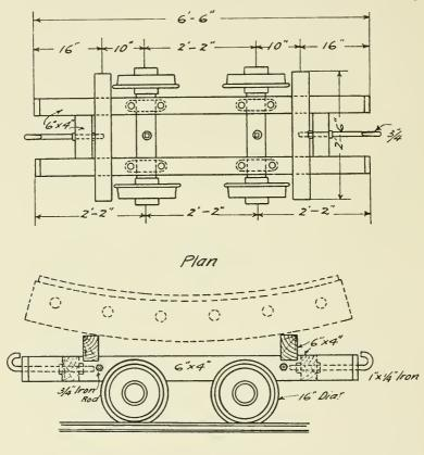
Fig. 87.—Car used for carrying segments of cast iron tunnel lining. Tunnel (A-18).
