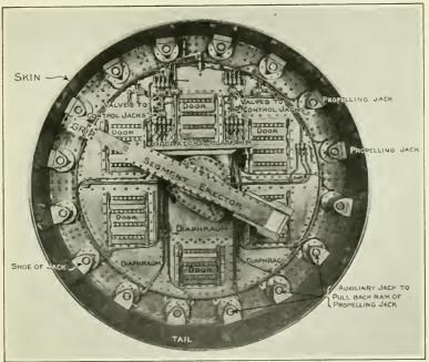
Fig. 82.—The parts of a shield. Rear elevation.
