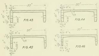
Fig. 43.—Tentative cast iron cross section to meet requirements of example.
