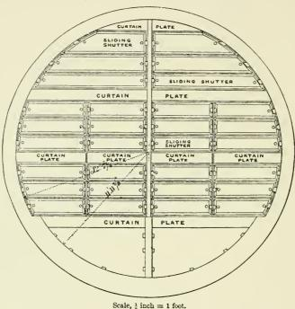
Fig. 75.—Blackwall tunnel (E-7) shield. Face shutters. (From *Proc. Inst. C. E.*, vol. 130.)
