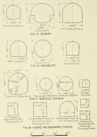
Fig. 15.—Cross sections of sewer tunnels. Fig. 16.—Cross sections of aqueduct tunnels.
