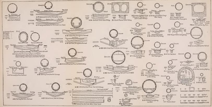
FIG. 20.-Cross sections and profiles of some tunnels which have been driven by shields under waterways.
