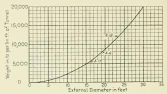
Fig. 38.—Cast iron lined tunnels in Hudson River silt. Relationship between diameter and weight of cast iron.
