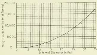
Fig. 36.—Cast iron lined tunnels in London clay. Relationship between diameter and weight of east iron.
