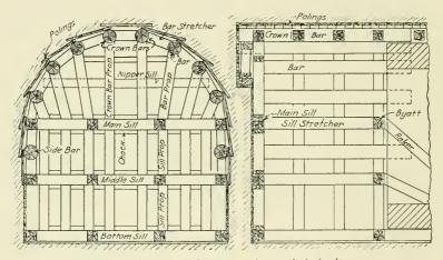
Fig. 4.—The English system of tunnel timbering.
