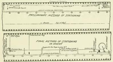
Fig. 161.—Two methods of "stationing" in a tunnel. The upper is a rapid method giving a good approximation as the work of tunnel driving proceeds. The lower is a slower but more accurate method for use after the driving period is over.
