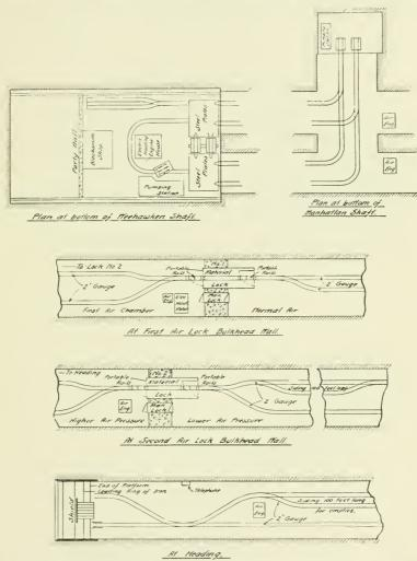
Fig. 86.—Plans of tracks, sidings and switches in a compressed air tunnel (Λ-18).
