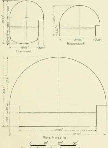
Fig. 19.—Cross sections of canal tunnels.
