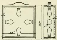
Fig. 157.—Tunnel light-box with electric lights screened by tracing cloth.
