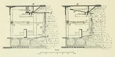
Fig. 113.—Blackwall Tunnel (E-7). Method of work in bottom pockets in wet gravel (or "ballast"). (Courtesy, of W. C. Copperthwaite.)
