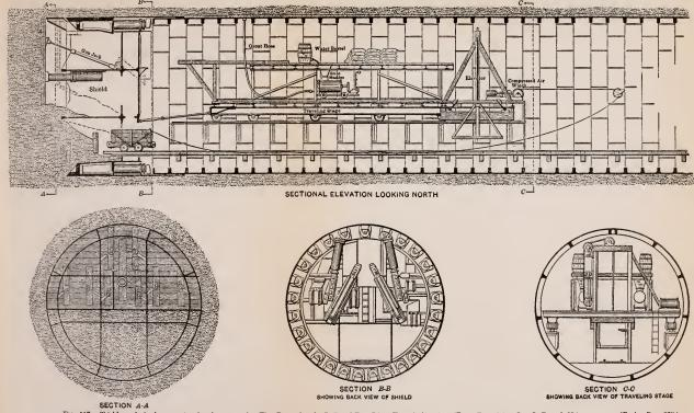
Fig. 117,-Shield work in loose water bearing ground. The Penneylvania Railroad East River Tunnele (A-19). (From Trons, Am. Soc C. E., vol. 68.)
