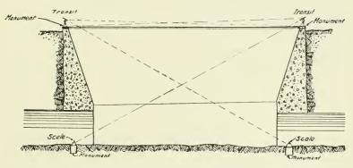
Fig. 155.—Method of transferring line from surface to tunnel where the shaft is on the line of the tunnel and large enough to enable the tunnel monument to be visible from the top of the shaft on the opposite side.
