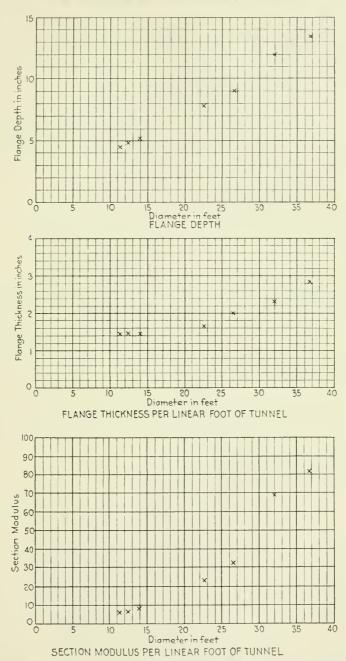
Fig. 40.—Cast iron linings in London elay. Relationship between diameter of tunnel and flange depth, flunge thickness per linear foot of tunnel and section modulus per linear foot of tunnel.
