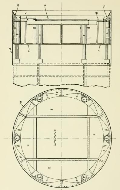
Longitudinal Section. Fig. 66.—Greathead shield for small diameter tunnel in London clay. Elevation of Shield—Rear View.
