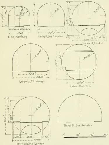
Fig. 12.—Cross sections of highway tunnels—one- and two-way.
