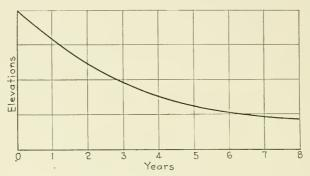
Fig. 138.—General downward movement of shield-driven tunnel in mud. This movement becomes slower and slower as years go by.
