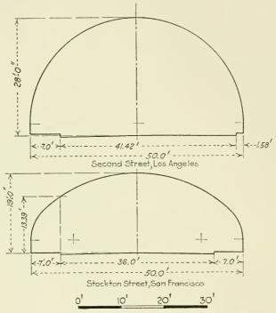
Fig. 13.—Cross sections of highway tunnels—four-way.
