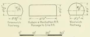
Fig. 14.—Cross sections of footway tunnels.
