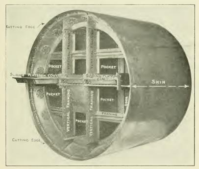
Fig. 84.—The parts of a shield. Front perspective.
